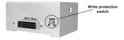
Once the DVI Detective is programmed and working, you can write protect the unit to prevent an accidental overwrite. This is done by simply moving the write protect switch to the D (write disabled) position. By default, the unit is shipped in the E (write enabled) position. This is done so that the unit is ready to be programmed right out of the box. Whenever the unit is going to be programmed, make sure that the switch is in the "E" position, otherwise the procedure will fail.
